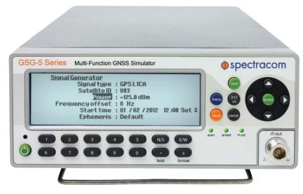
The GSG-51 is a GNSS signal generator that emulates a single GNSS signal. The main application is a simple but very fast manufacturing test, to assure that the assembly is correct, that the antenna is properly connected, and that the receiver can receive and identify a satellite signal.
