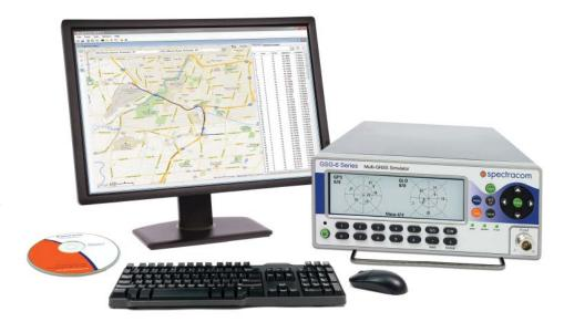
any GNSS constellation, any particular signal. Or some of these channels can be used for SBAS simulation of EGNOS, WAAS, GAGAN, or MSAS satellites, or for simulating multipath or interference. If more channels are required, simply synchronize two or more units via the external 1PPS sync signal to generate 128, 256, or more channel simulation. Some restrictions apply.
