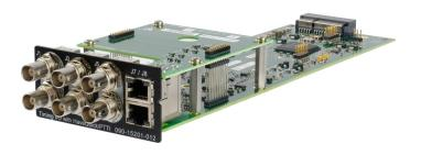
The Standard S650 Timing I/O module is outfitted with two RJ48 connectors to support RS422 PTTI Outputs. Additionally, HaveQuick timecodes are supported as inputs and outputs. All circuitry on the module has been upgraded to support 5V and 10V input and output pulses common to HaveQuick and PTTI signals. Due the tremendous range of signaling options for this module, the FlexPort license is required.
